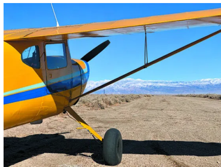
Tamer Abubakr put tundra tires on his Cessna 120 shown here. Coupled with a 135-HP Lycoming O-290-D, it's a heck of a good performer
