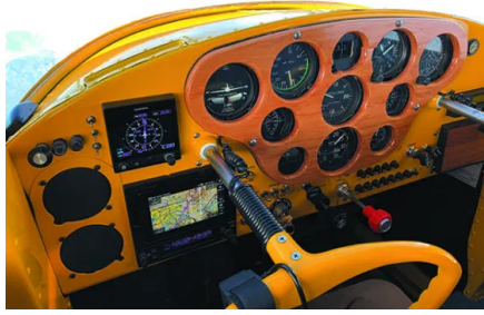
It's small, but the custom panel in Tamer Abubakr's Cessna 120, is a work of art. That's a Garmin G5 electronic flight instrument, a Garmin portable GPS and a Garmin comm radio.
