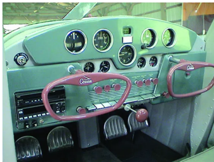
This one has been retrofitted with a basic radio and transponder.
